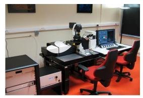
Microscope confocal Gated-STED (TCS SP8 Leica\*)
